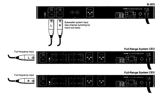
All Meyer Sound loudspeaker systems are designed to be used with their respective Control Electronics Units. When such systems are used with Meyer Sound subwoofers, the B-2EX input should be connected in parallel with the full-range (biamplified) system input as shown in the diagram above. Where mono
